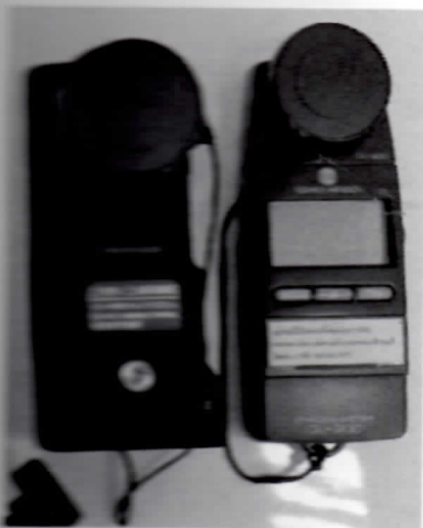
Fig 2. Measurement equipment and set up distance (1) Minolta CL500 and CL200 (2) Equipment set up inside the booth
