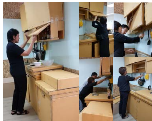
Figure 9 The first kitchen mock-up test scale 1:1
