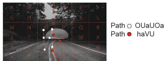
Fig. 3. Example of scan-path analysis showing two scan-paths over grid types, and how the grid layout affects the letter sequence describing the path.
