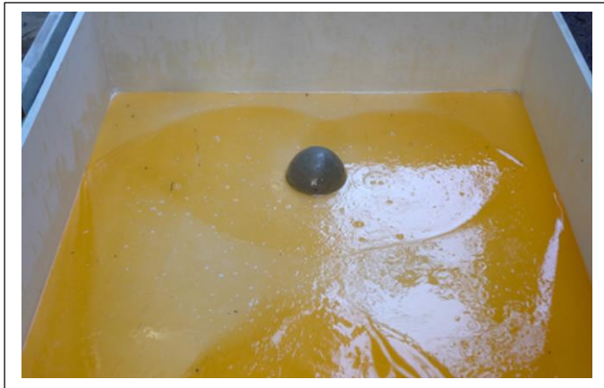
Fig. 20, Miniature Wave Tank, Wave Interference Experiment.
