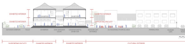
Figure 8 Sectional drawing of Phuket Thai Hua Museum showing interior-exterior connection (Image by authors)
