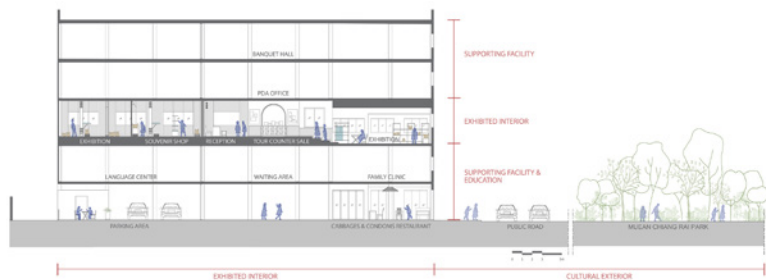
Figure 11 Sectional drawing of the PDA building shows the location of interior programs. (Image by authors)
