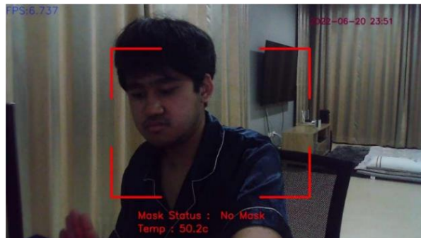
Fig. 7. Screen after tapping the IR Sensor and starting the screening of users with a fever (temperature above 37.5 Celsius) and not wearing a hygienic mask.
