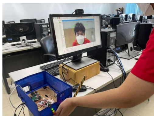
Fig. 8. Temperature measurement system test body from the screening system
